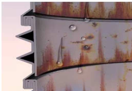
Conventional folded seam joints can loosen under compressive loads allowing condensates to enter
